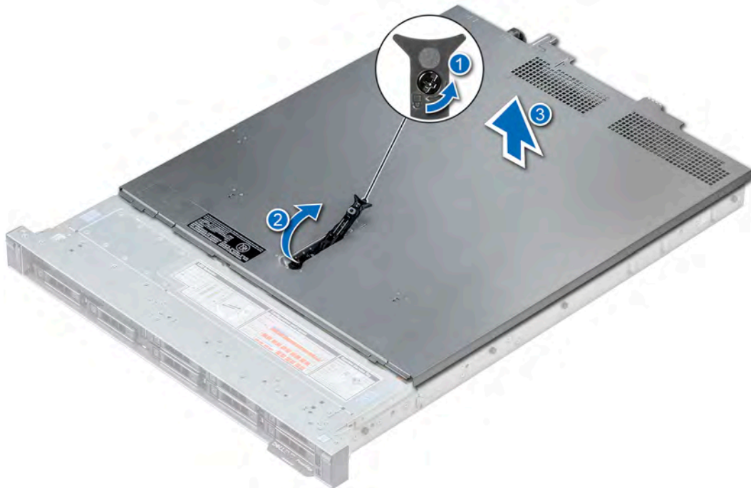
Figure 19. Removing the system cover
