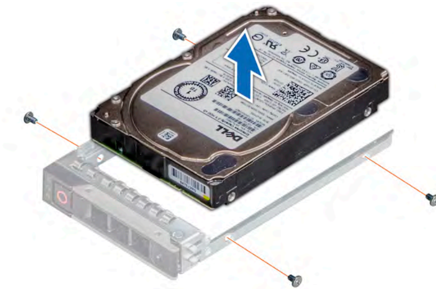
Figure 38. Removing the drive from the drive carrier
