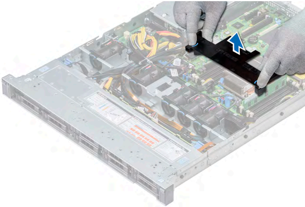
Figure 24. Removing the air shroud
