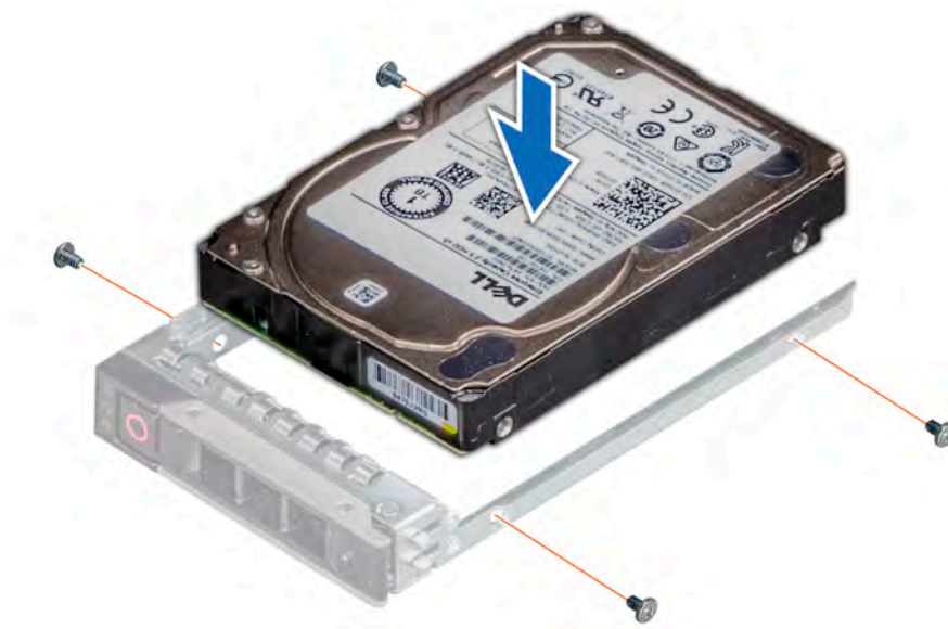
Figure 39. Installing a drive into the drive carrier
