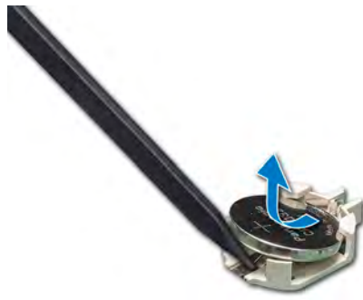
Figure 93. Removing the system battery
