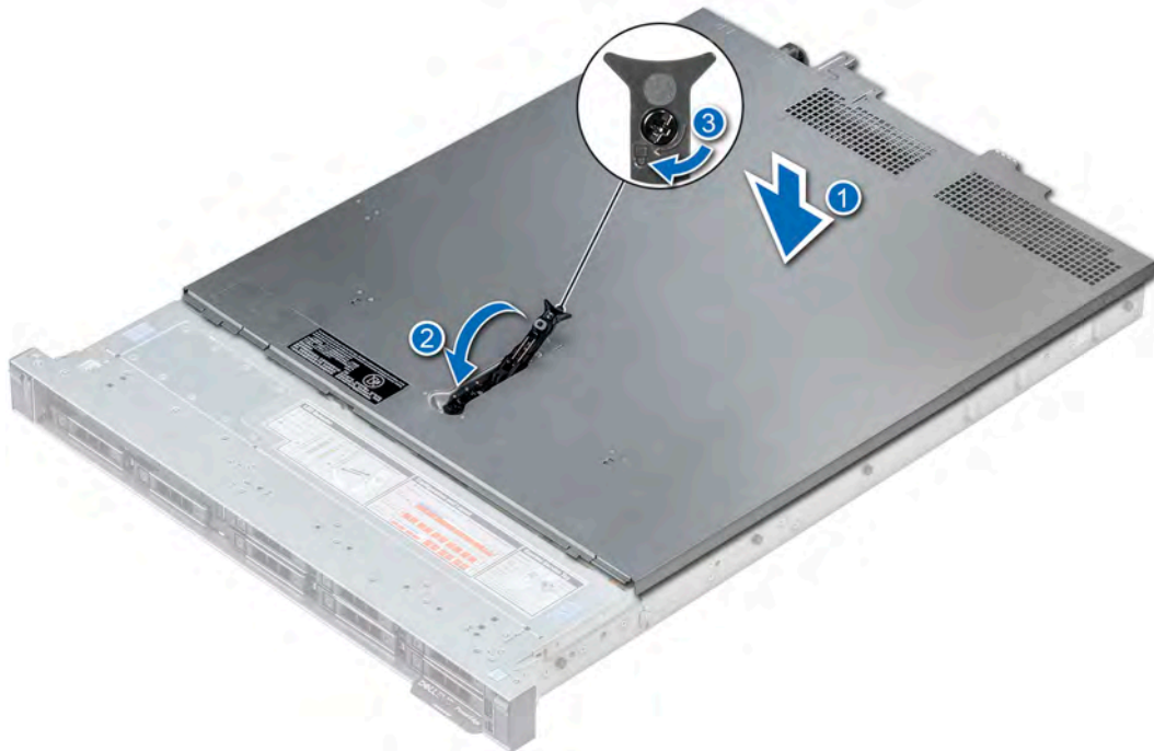
Figure 20. Installing the system cover
