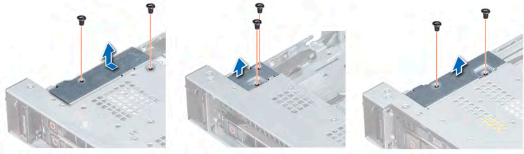
Figure 105. Removing the cable cover
