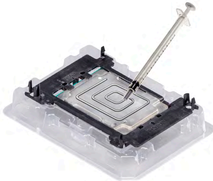
Figure 47. Applying thermal grease on top of the processor
