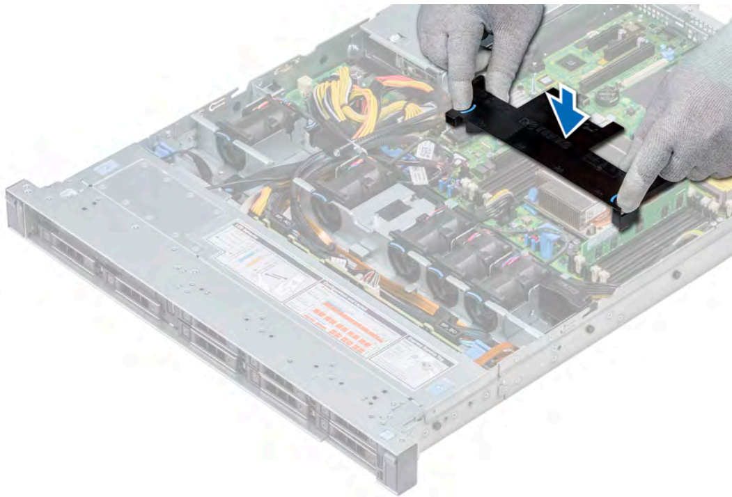
Figure 25. Installing the air shroud
