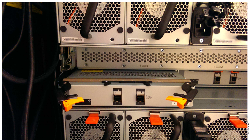
Figure 89. Removing the expansion canister
