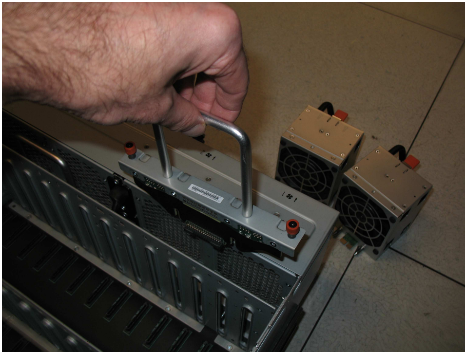
Figure 96. Remove the FIB from the chassis
