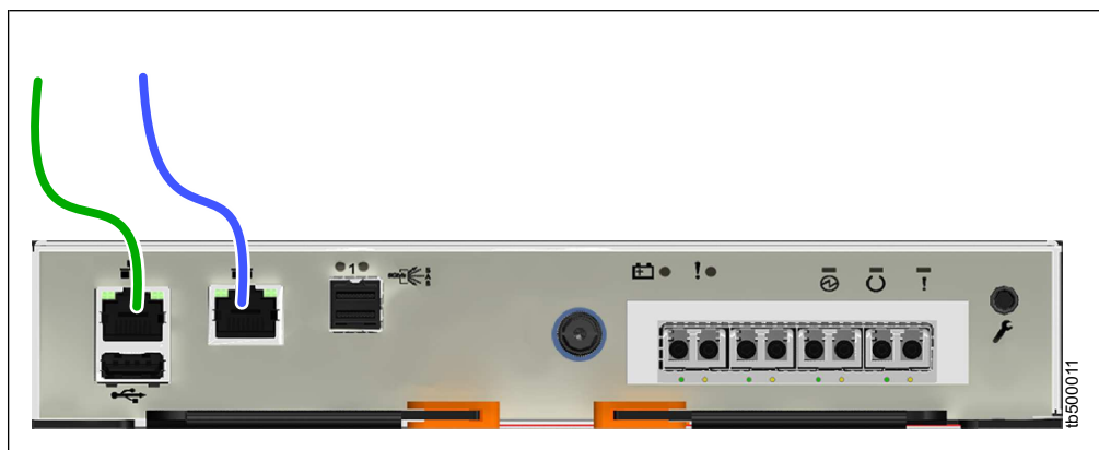
Figure 110. Connecting the Ethernet cables to a Storwize V5010 system
