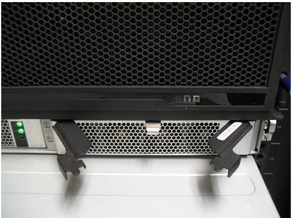
Figure 64. Install the power supply
