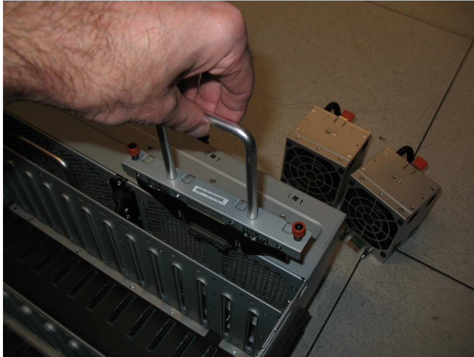
Figure 74. Insert the new FIB in the chassis
