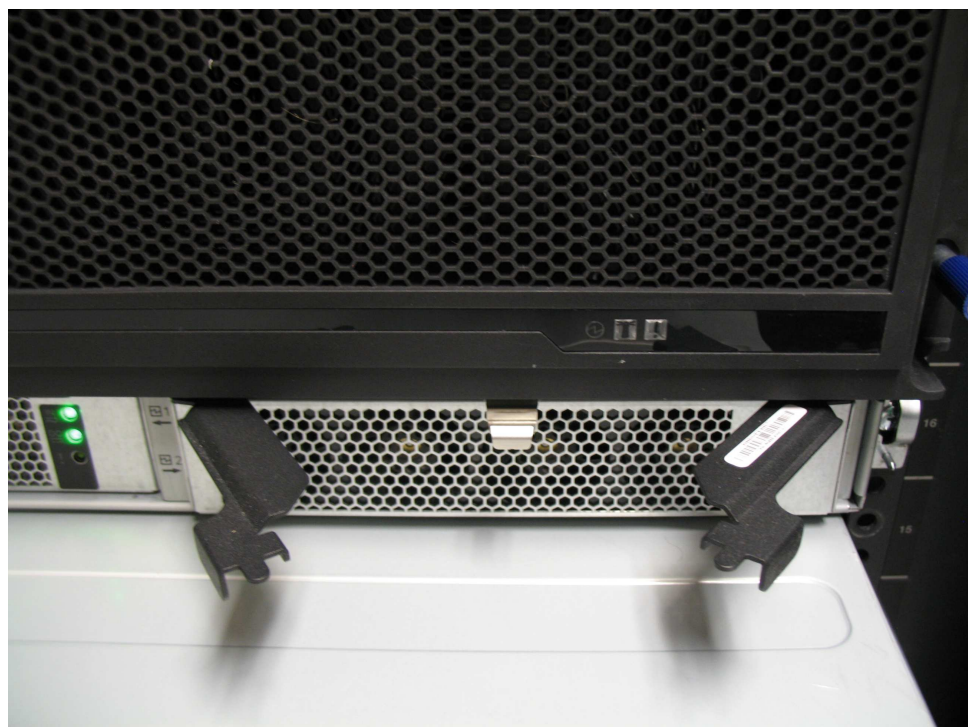
Figure 78. Releasing the power supply handles
