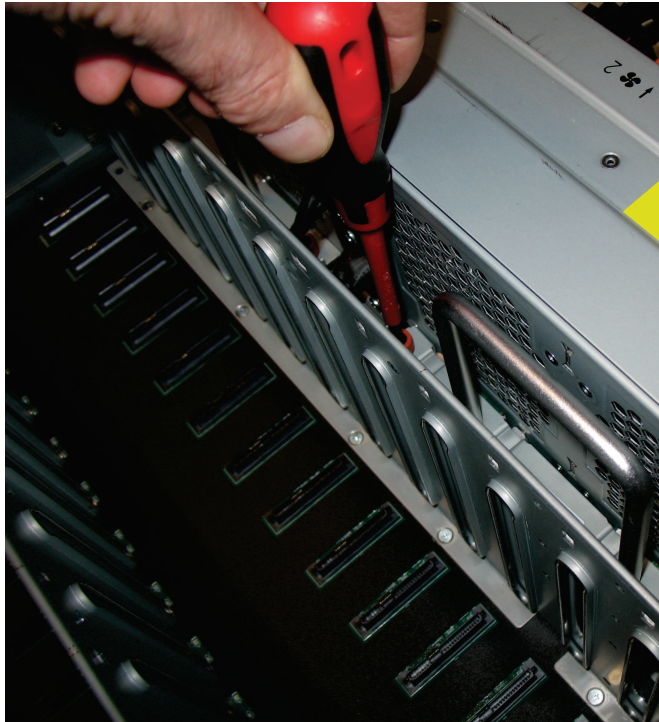
Figure 95. Loosen the FIB screws
