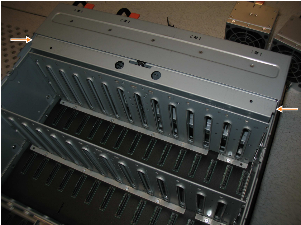
Figure 76. Replace the FIB cover
