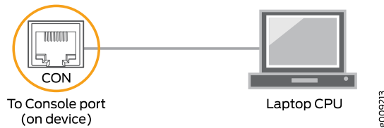
Figure 20: Connecting the MX150 Directly to a Management Console
