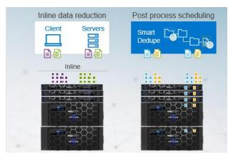
asynchronous deduplication. After duplicate blocks are discovered, SmartDedupe moves a single copy of those blocks to a special set of files known as shadow stores. During this process, duplicate blocks are removed from the actual files and replaced with pointers to the shadow stores.
