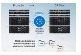
Performance of SynclQ include incremental transfer where only changed blocks are replicated, snapshot integration, bandwidth metering, monitoring, throttling and flexible scheduling. For availability, SynclQ jobs can be configured for alerting and logging along with failure and recovery.
