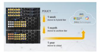
CloudPools software provides policy-based automated tiering that lets you seamlessly integrate with the cloud as an additional storage tier for the cluster. This allows you to address rapid data growth, reduce storage costs and optimize data center storage resources by using the cloud for frozen data. In this way, your more valuable storage may be used for more active data and applications, while frozen data may be retained at minimum cost for compliance, historical or other business reasons.
