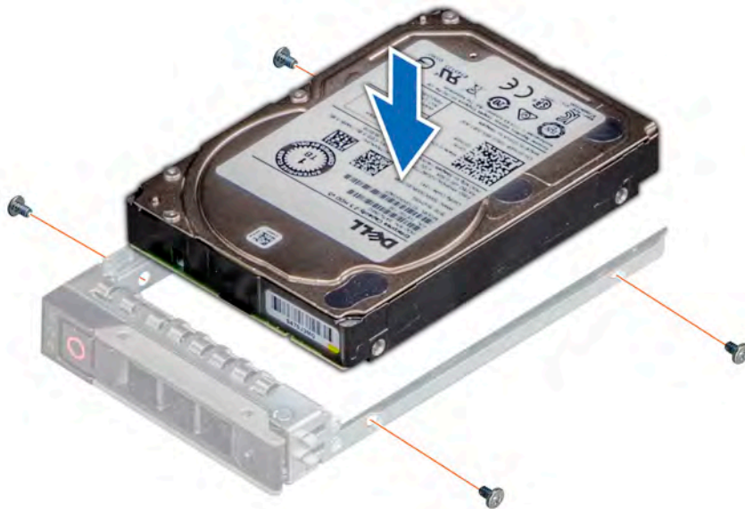
Figure 41. Installing a drive into the drive carrier
