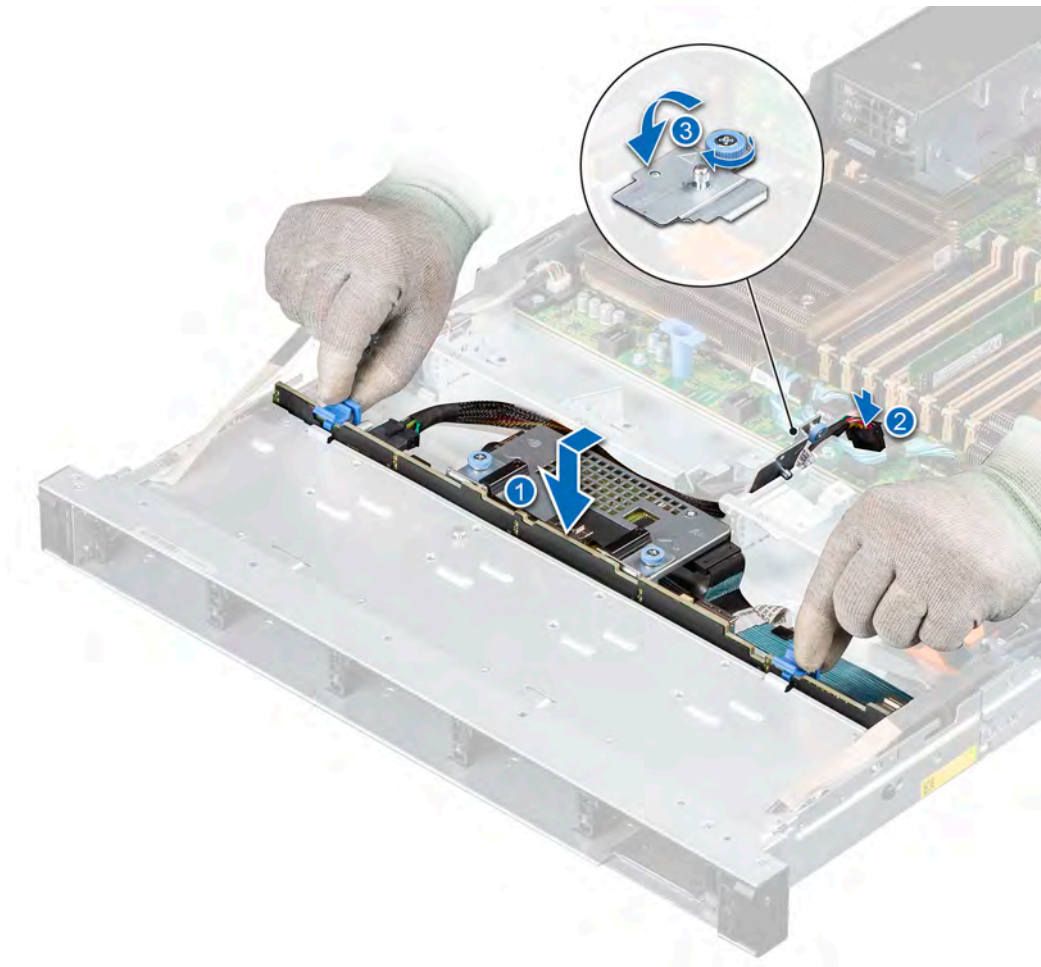
Figure 46. Installing the drive backplane
