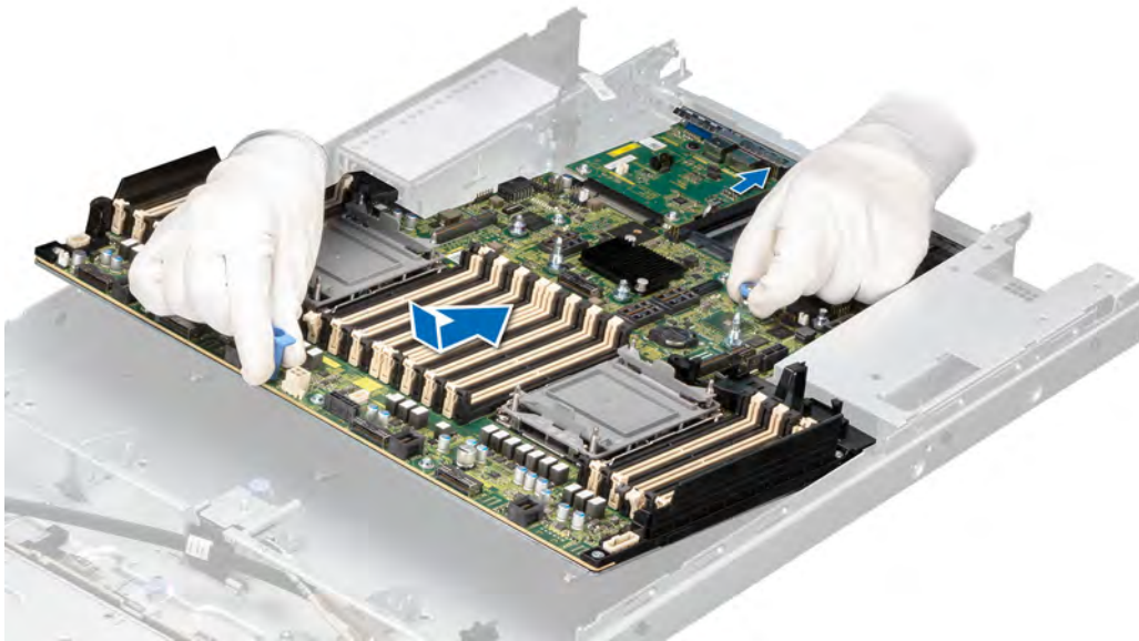
Figure 129. Installing the system board
