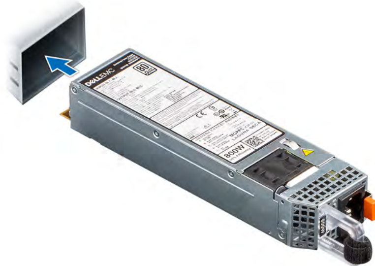
Figure 123. Installing a power supply unit
