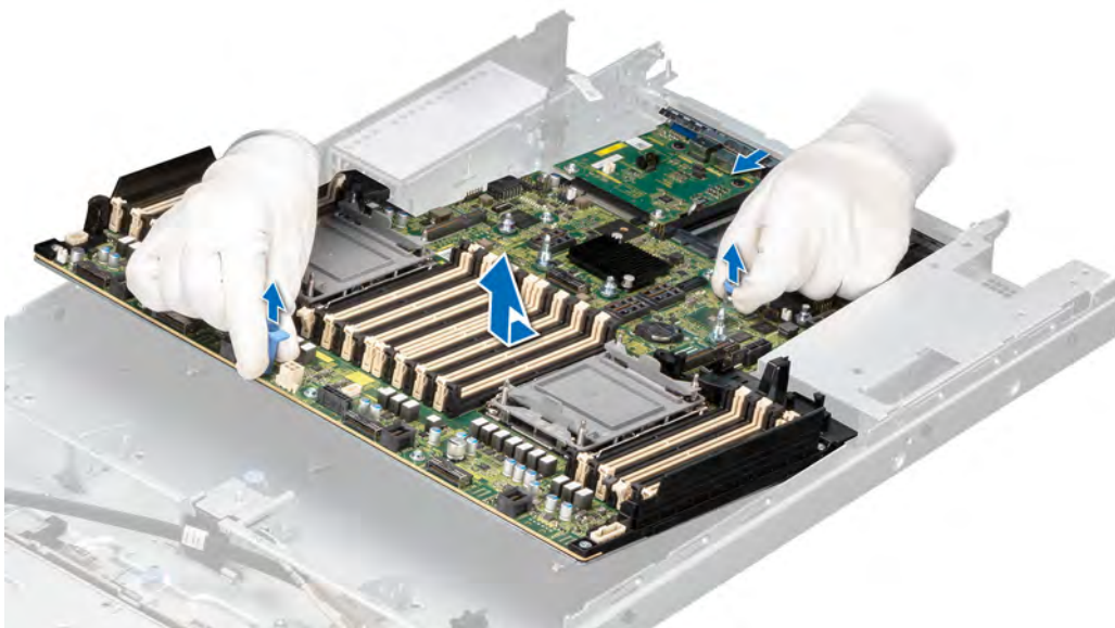
Figure 128. Removing the system board
