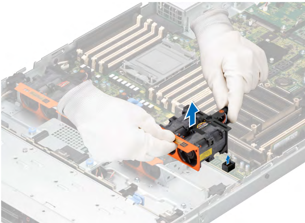
Figure 34. Removing a cooling fan module
