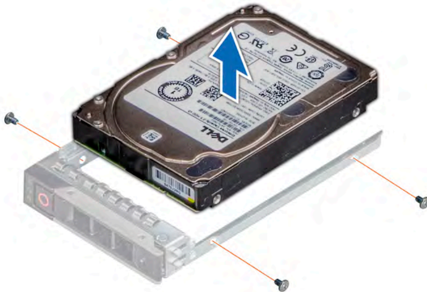
Figure 40. Removing the drive from the drive carrier
