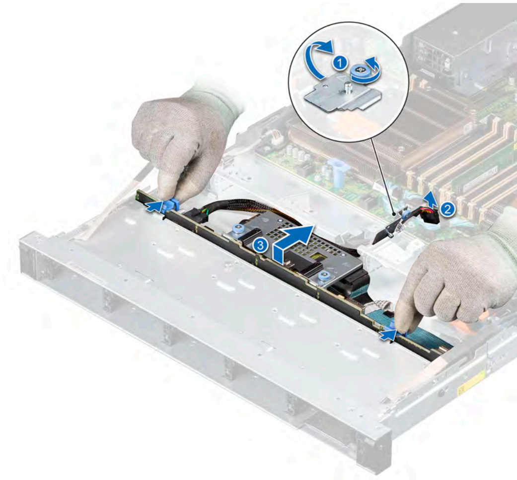
Figure 45. Removing the drive backplane
