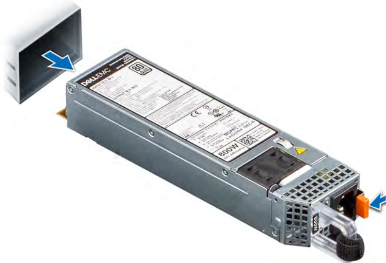
Figure 122. Removing a power supply unit
