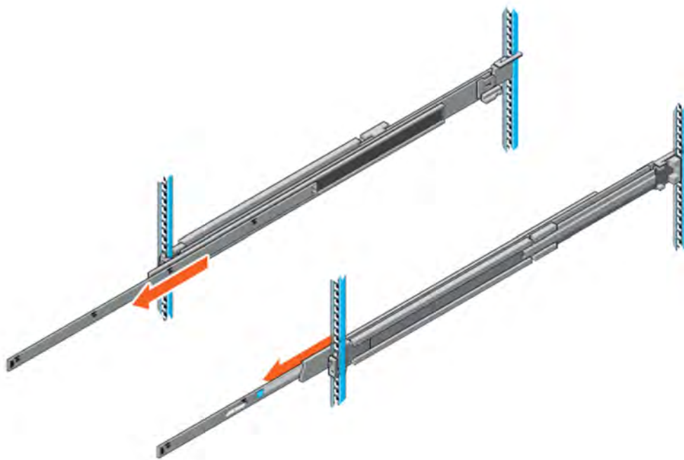
Figure 32. Pull out inner rail
