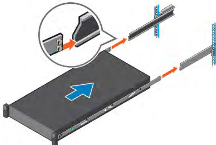
Figure 37. Install system into the extended rails
