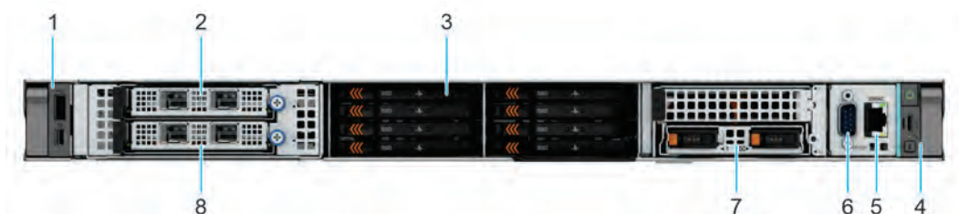
Figure 2. Front view of 8 x EDSFF E3.S drive system with front I/O configuration
