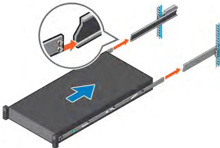
Figure 30. Install system into the extended rails
