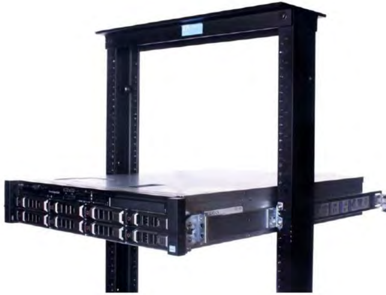
Figure 39. Static rails in 2-post center mount configuration
