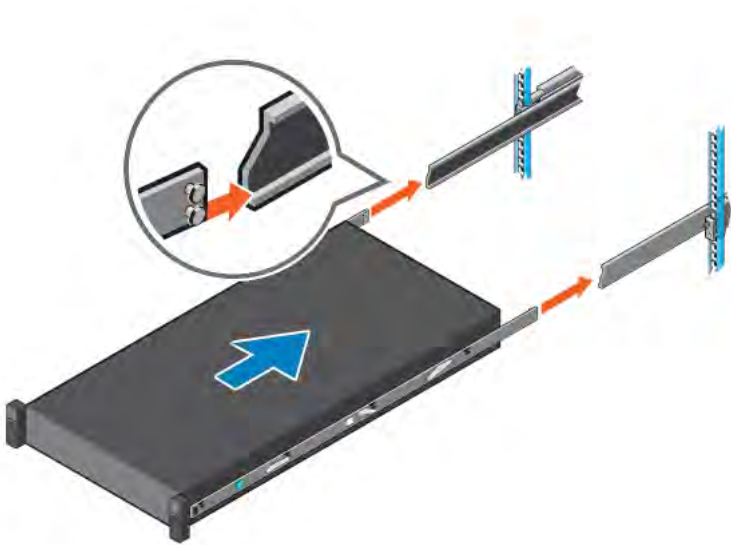
Figure 48. Install system into the extended rails
