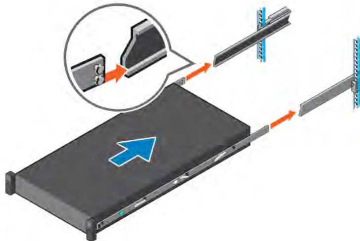
Figure 34. Install system into the extended rails
