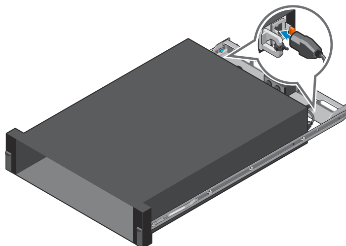
Figure 38. Connecting power cable to system
